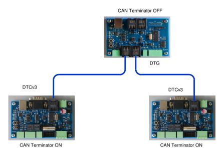
To connect two DTC modules to a DTG, repeat the game from section 3.2. The difference here is: Since the DTG is connected with both RJ45-CAN connectors, it is NOT on the end of the CAN bus and so the CAN terminator is OFF.
