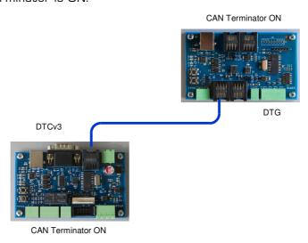
**NOTE** that power for the DTG module is supplied by the DTCv3 module and that the DTCv3 is set to supply power to the CAN bus. If you connect a USB cable from your PC to the DTG module, the blue LED on the USB interface will light up. However, the DTG only works when the red LED on the DTG module also lights up!
