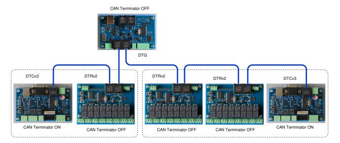
The diagram above shows a grouping, which DTR modules belong to which DTC. **NOTE:** This grouping is determined solely by configuration and is not influenced by the order in which you connect the modules.
